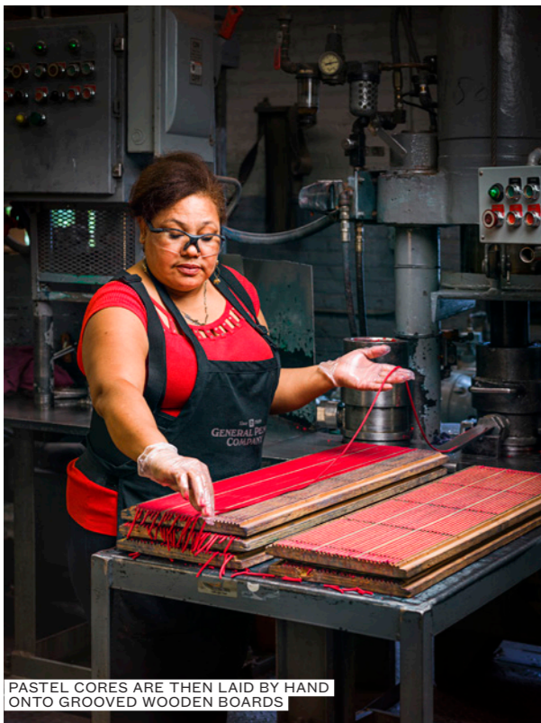
THE PASTEL CORES ARE FRAGILE AND MUST BE PLACED CAREFULLY INTO PRE-GLUED CEDAR SLATS
